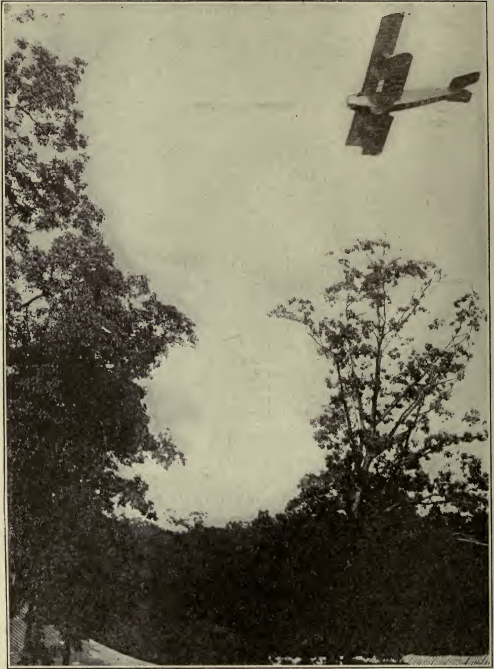
A good illustration of how an airplane may drop to dangerous levels when coming out of an aerial fountain
