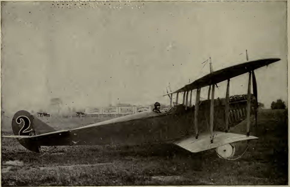
An airplane of the "tractor" type, so called because the propeller is attached to the front, pulling the machine through the air
