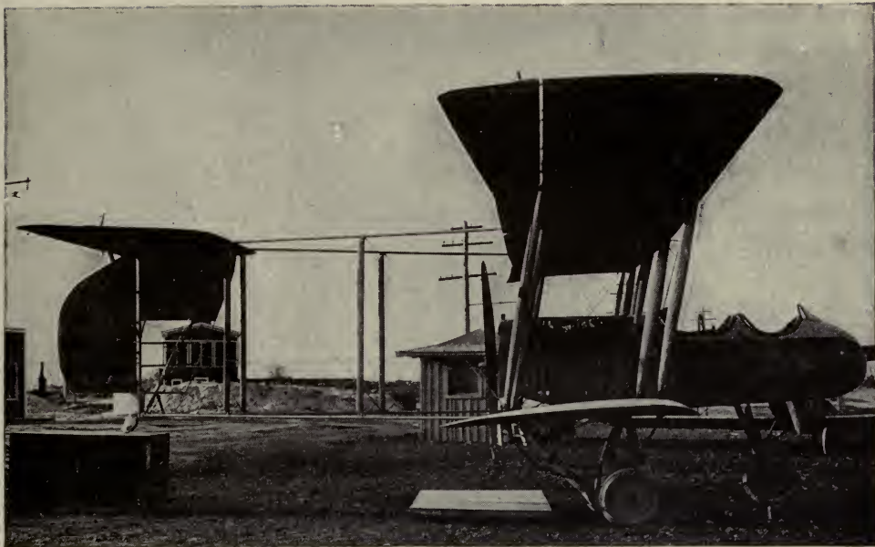
A "pusher" biplane with the propeller back of the wings or main lifting surfaces and the pilot's seat directly in front
